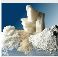
RUBITHERM® RT is a pure PCM, this heat storage material utilising the processes of phase change between solid and liquid (melting and congealing) to store and release large quantities of thermal energy at nearly constant temperature. The RUBITHERM® phase change materials (PCM's) provide a very effective means for storing heat and cold, even when limited volumes and low differences in operating temperature are applicable.
