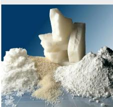
RUBITHERM<sup>®</sup> RT is a pure PCM, this heat storage material utilising the processes of phase change between solid and liquid (melting and congealing) to store and release large quantities of thermal energy at nearly constant temperature. The RUBITHERM<sup>®</sup> phase change materials (PCM's) provide a very effective means for storing heat and cold, even when limited volumes and low differences in operating temperature are applicable.
